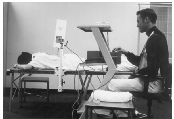
FIGURE 32-3. The Stiffness Assessment Machine (SAM) being used to test posteroanterior stiffness at L3. (Reproduced with permission from Squires MC, Latimer J, Adams RD, Maher CG. Indenter head area and testing frequency effects on posteroanterior lumbar stiffness and subjects' rated comfort. Manual Ther 2001;6:40-47.)
