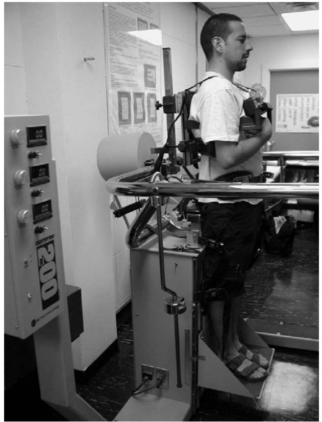
FIGURE 32-8. The B200 Triaxial Isoinertial Dynamometer (Isotechnologies, Inc., Hillsborough, NC) is used for isoinertial trunk muscle strength testing.
